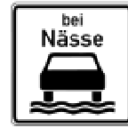
Found directly under a speed limit sign. Indicates speed limit in effect ONLY when wet
